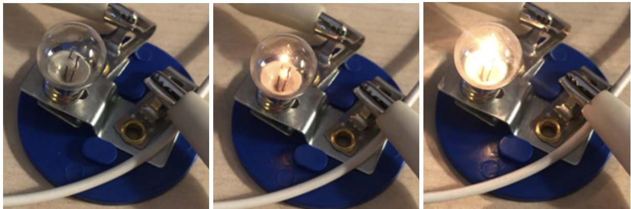
Figure 29: Light Bulb Sweeping Through Brightness Levels with Arduino PWM
